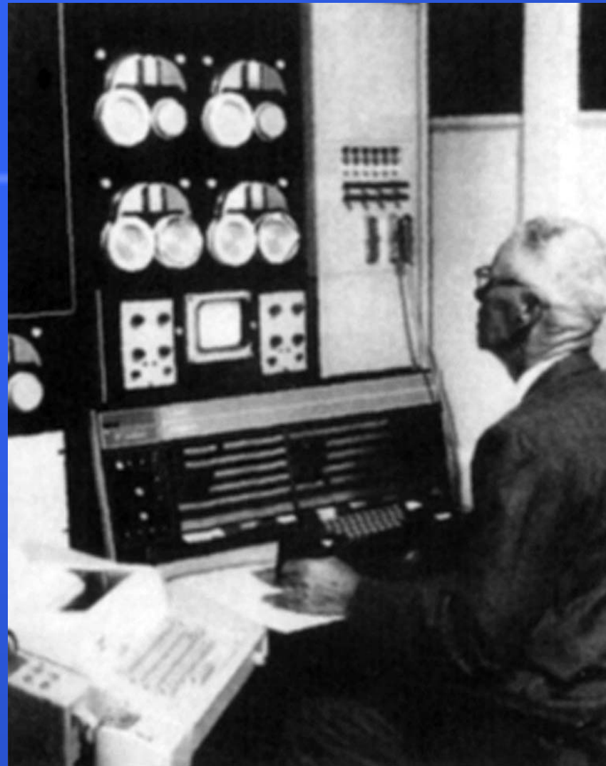
Fig. 6.1 The LINC (Laboratory Instrument Computer) in use in a medical interview in 1968. (Reproduced from Slack WV, Van Cura LJ. Patient reaction to computer-based medical interviewing. Computers in Biomedical Research 1968; 1:527-531 with permission.)
